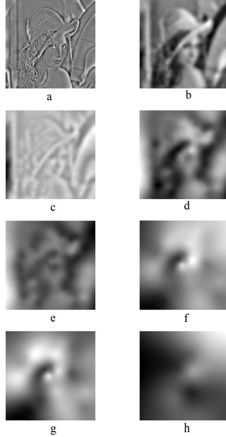
Figure 2. a) First IMF, b) first residue, c) second IMF, d) second residue, e) third IMF, f) third residue, g) fourth IMF, h) fourth residue.
