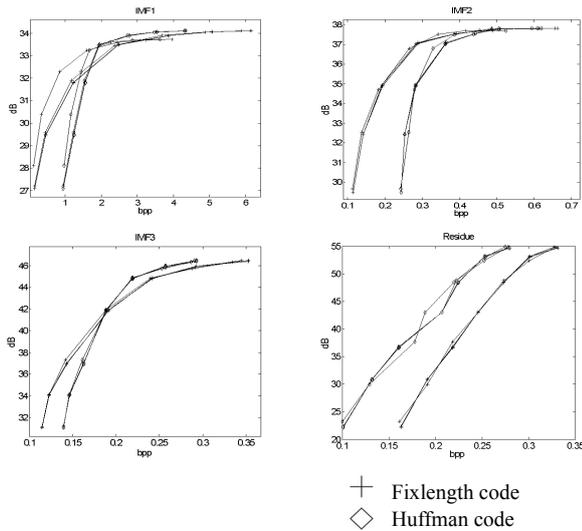
Figure 3. VSDCTEMD Coding result of Detail two. Zero zone=1, 10, 20 quantization varies from 256 levels down to 8 levels
