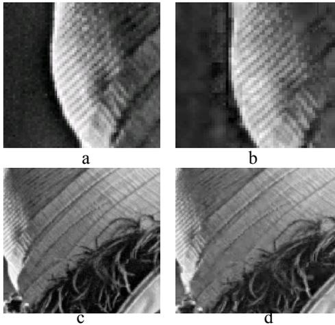
Figure 5. VSDCTEMD. a) Detail one original, b) Detail one image reconstructed to 28.27 dB using 4.79 bpp. c) Detail two original, d). Detail two image reconstructed to 30.76 dB using 3.56 bpp.
