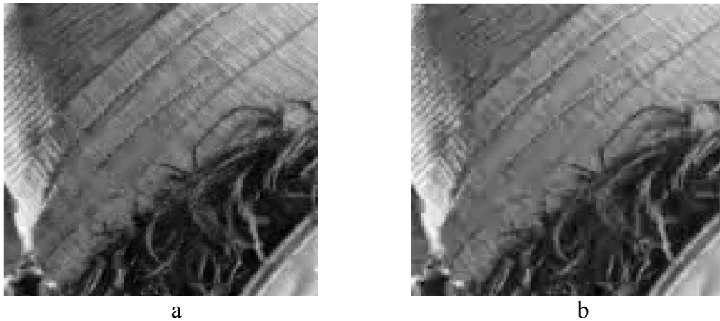
Figure 9.21. Result of coding Detail two by VSDCTEMD in first IMF and DCT threshold coding on first residue. a) 1.2788 bpp 30.0208 dB, b) 0.69 bpp 28.88 dB
