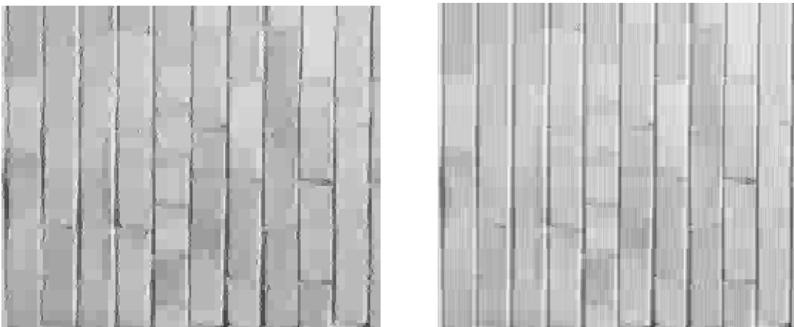
Figure 3.32. To the left: brickwall coded with SPIHT at 0.0631 bpp, PSNR=22.0631. To the right: brickwall coded with constrained CWP at 0.0624 bpp, PSNR=22.7652
